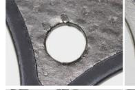
Worn, uneven cut tools to save cost. Poor sealing ability.
