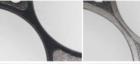
Separated fire rings to save tooling cost. Prone to compression leaks over-time.
